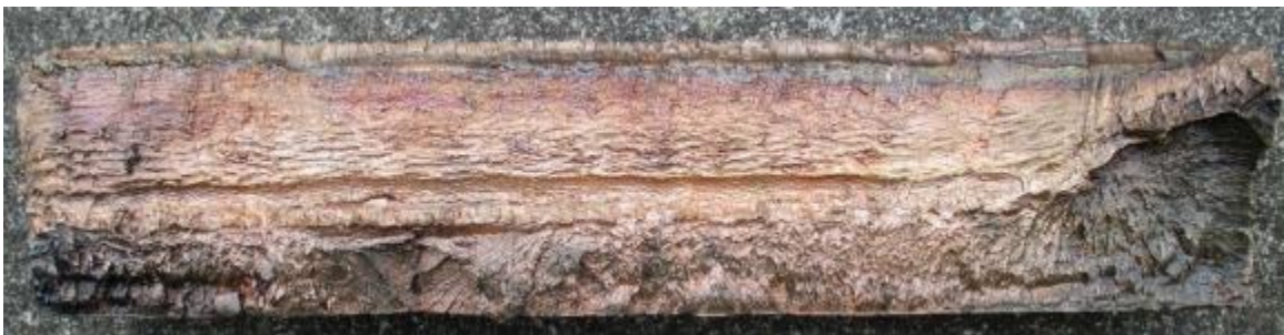
Figure 6.1. Target typical of an LSC test. Note that this target fractured completely and did not need to be cut post-test
