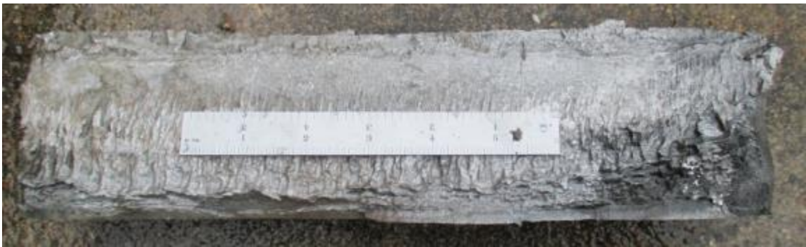
Figure 6.6. Aluminum target that was recovered after 2,000 gr/ft. LSC penetration
